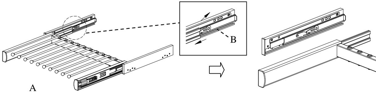
Step 2: If the cupboard is 16mm thickness, washer can be added to the aluminum spacer.
