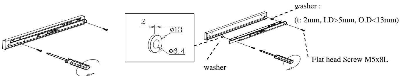
Step 3: Screw aluminum spacer to the partition wall.
