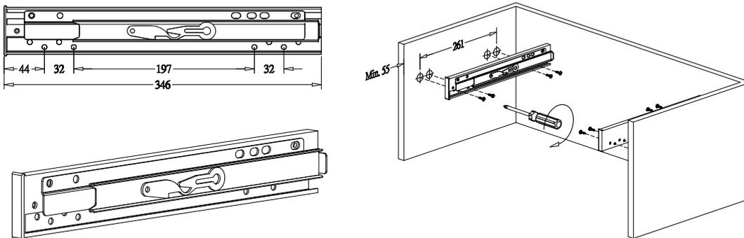
Step 4: Join outer slide together with the inner channel.
